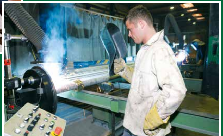
Mechanised welding line
